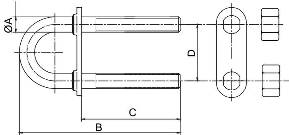
We advise a working load of 1,000 lbs for 3/8" stock diameter and 2,000 lbs for 1/2" stock diameter. Please note for ABYC H-40 section 40.7.1.3 "A bow eye intended for the use of trailering or being towed (e.g., a tender), shall be able to accommodate a direct tension pull, in the forward direction, of one half of the boat weight."
