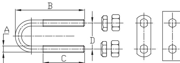
We advise a working load of 1,000 lbs for 3/8" stock diameter and 2,000 lbs for 1/2" stock diameter. Please note for ABYC H-40 section 40.7.1.3 "A bow eye intended for the use of trailering or being towed (e.g., a tender), shall be able to accommodate a direct tension pull, in the forward direction, of one half of the boat weight."
