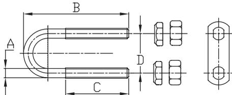
We advise a working load of 1,000 lbs for 3/8" stock diameter and 2,000 lbs for 1/2" stock diameter. Please note for ABYC H-40 section 40.7.1.3 "A bow eye intended for the use of trailering or being towed (e.g., a tender), shall be able to accommodate a direct tension pull, in the forward direction, of one half of the boat weight."
